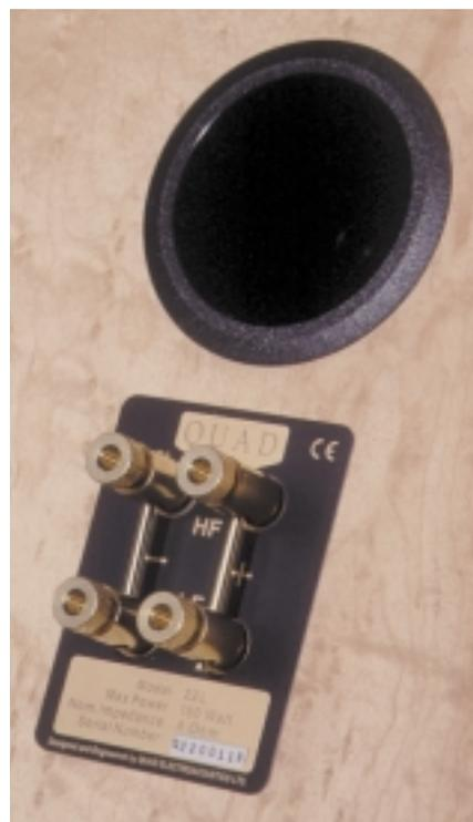
enclosure. It is split for bi-wiring, so four gold-plated 4mm socket/binding posts are fitted (linked with bars as supplied, for a conventional two-wire feed). Nominal impedance is 6 ohms, confirmed by my measurements, which revealed peaks at around 63Hz (14 ohms) and 16kHz (17.5 ohms); nowhere does it drop below 4 ohms. Sensitivity is quoted at 89dB for 2.83V at 1m.
